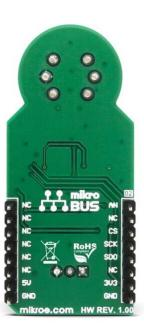
**Ozone 2** click carries an MQ131 sensor for Ozone (O<sub>3</sub>). The sensor outputs an analog voltage, which is converted by the onboard MCP3551 22-bit ADC converter or it is sent to the microcontroller via AN pin on the mikroBUS<sup>TM</sup>, depending on the position of ADC SEL. jumper. The click is designed to run on 5V power supply. It communicates with the target microcontroller over SPI interface or AN pin on the mikroBUS<sup>TM</sup> line.
