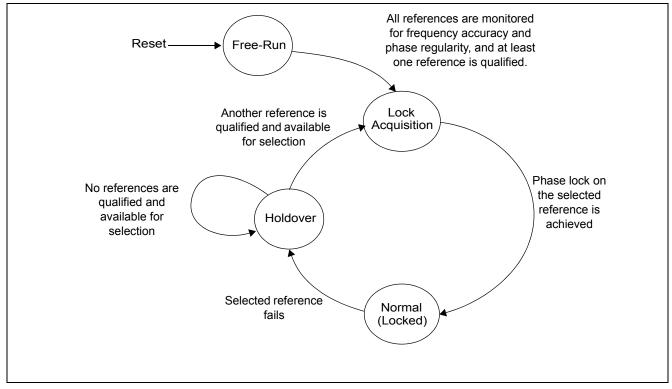
Figure 2 - Automatic Mode State Machine
