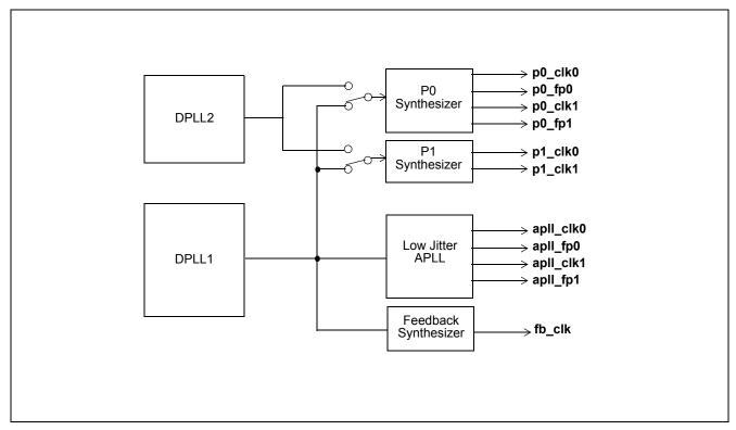
Figure 6 - Output Clock Configuration
