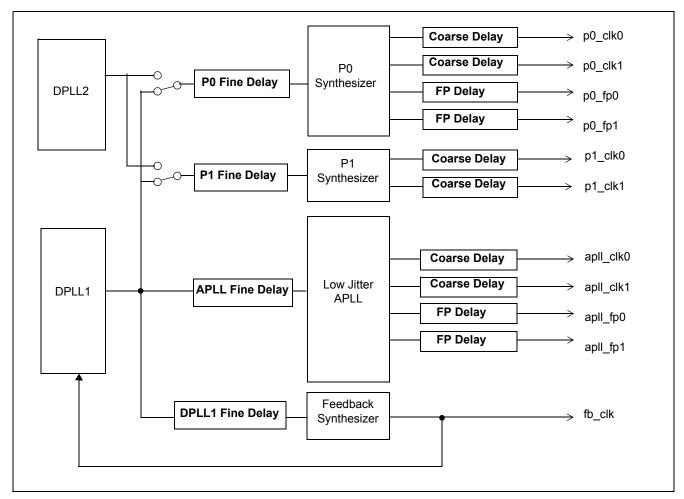
Figure 7 - Phase Delay Adjustments
