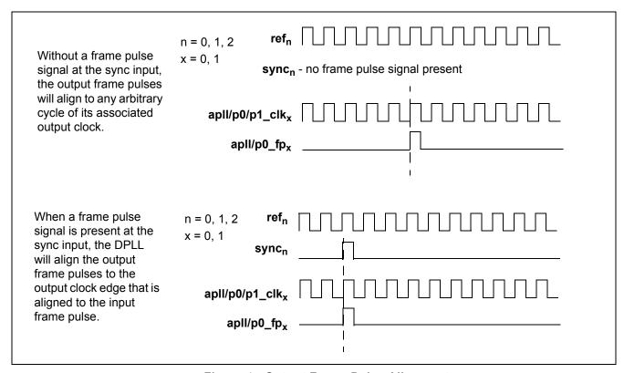
Figure 4 - Output Frame Pulse Alignment
