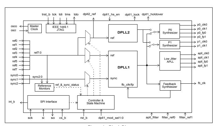
Figure 1 - Block Diagram
