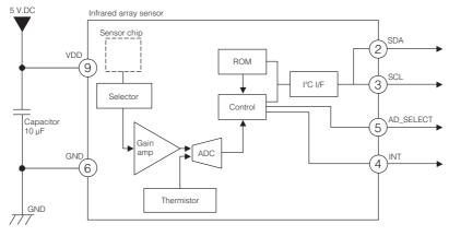
\* INT terminal 4 normally has same voltage as VDD. When interrupting, same as GND (0V)
