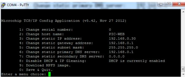
The third option allow you to change the board IP number. Just type 3, then enter the new IP compatible with your local network configuration. After that push ENTER and return to the main menu again.
