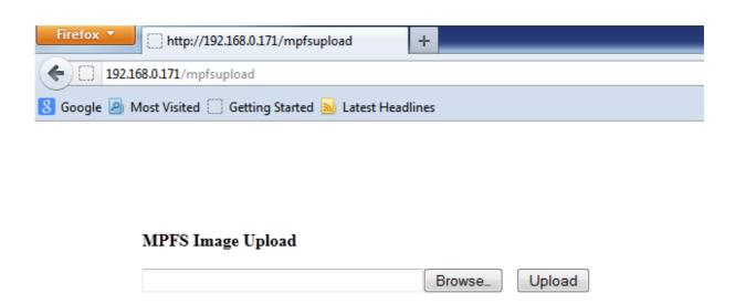
Click on the button "Browse\_" to select the "\*.bin" file you are about to upload. Select the image file in directory "PIC-WEB 5.42\TCPIP\Webpage MPFSImg prebuilt.bin" and press 'Upload'. Sit back and relax while the upload takes place and then navigate to the home page to behold the page just uploaded.
